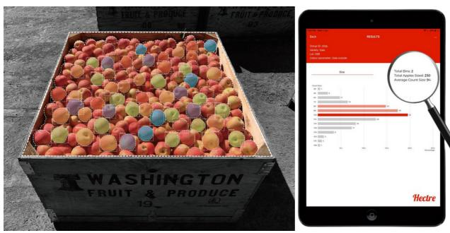
Hectre's mobile AI solution Spectre detecting and sizing pieces of fruit. High volume size sample results are available in seconds.
